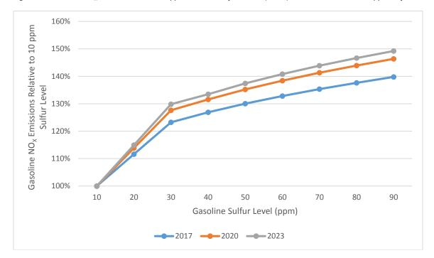
Figure 5-2. Gasoline  $NO_X$  Emissions at 10 – 90 ppm Gasoline Sulfur in 2017, 2020, and 2023 Relative to 10 ppm Sulfur Levels
