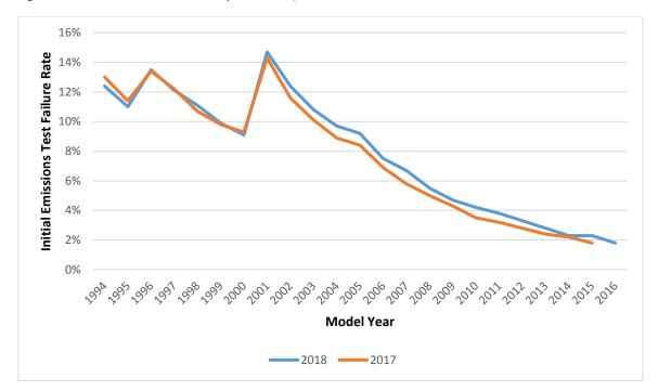
Figure 3-3. Emissions Test Failure Rate by Model Year, 2017 and 2018
