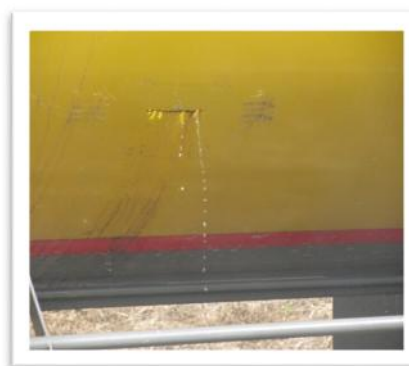
The leak in the side of the railcar.
