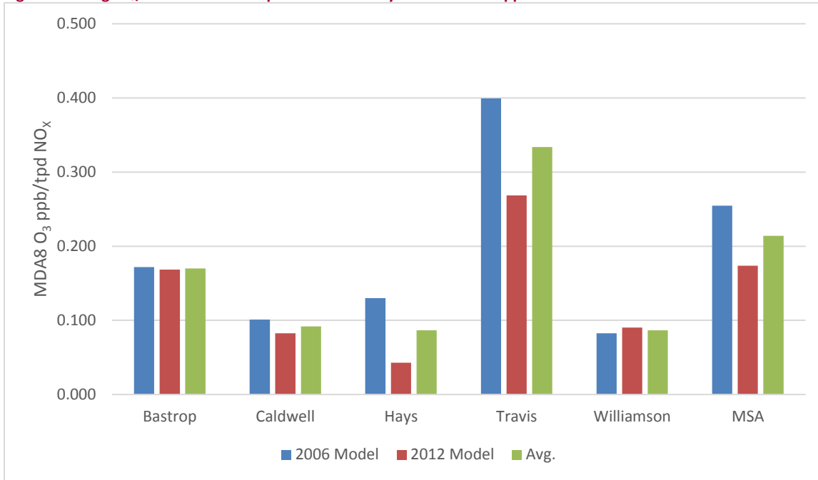
Figure 3-2. Avg. O 3 /NO x Ratios for Top 10 Modeled Days for 2017 ≥ 60 ppb at CAMS 3
